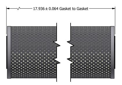
Pleated Paper Cartridge Part Number: PL718-10FPB Micron Rating: 10 Micron nominal Support structure: Plated Steel
